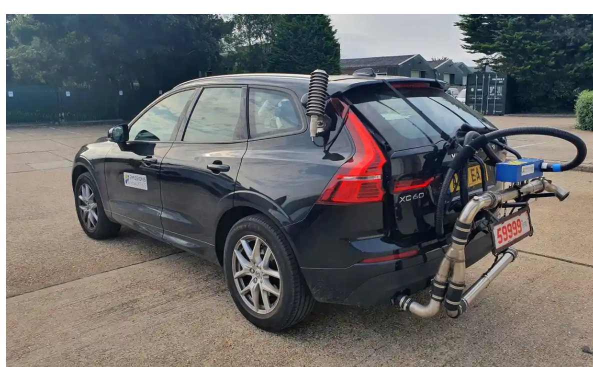
A Volvo hybrid car undergoes emissions tests for the campaign group Transport & Environment in 2021. Photograph: Emissions Analytics/Reuters
